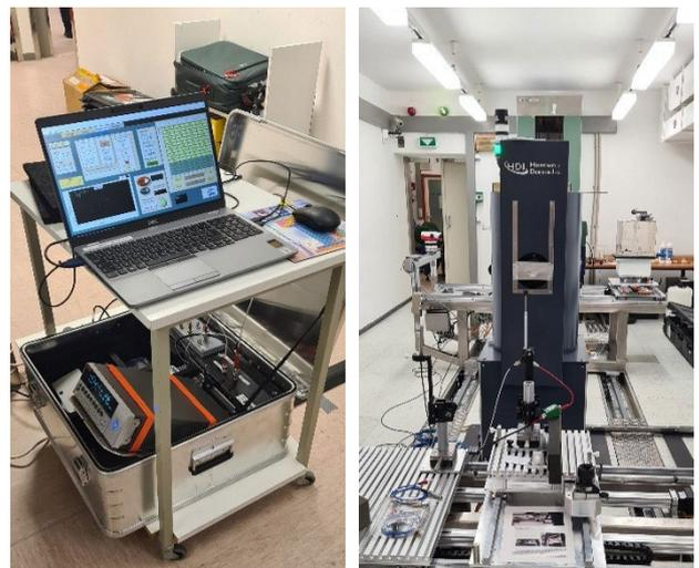
New BIPM measurement system (left) developed for the dosimetry K5 key comparisons using the  $^{137}\text{Cs}$  irradiator facility at the IAEA (right)
