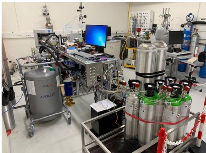
Isotope ratio Mass Spectrometer facility for comparison of pure CO<sub>2</sub> and CO<sub>2</sub> in air isotope ratio standards
